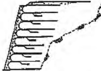
F) SLOPING GUNITE OR STRUCTURAL FACING
