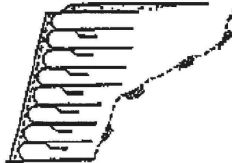
F) SLOPING GUNITING OR STRUCTURAL FACING
