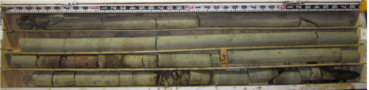
SHP MP 9.3 Boring B-2: Box 1 of 3 (15.0 to 30.0 ft bgs)
