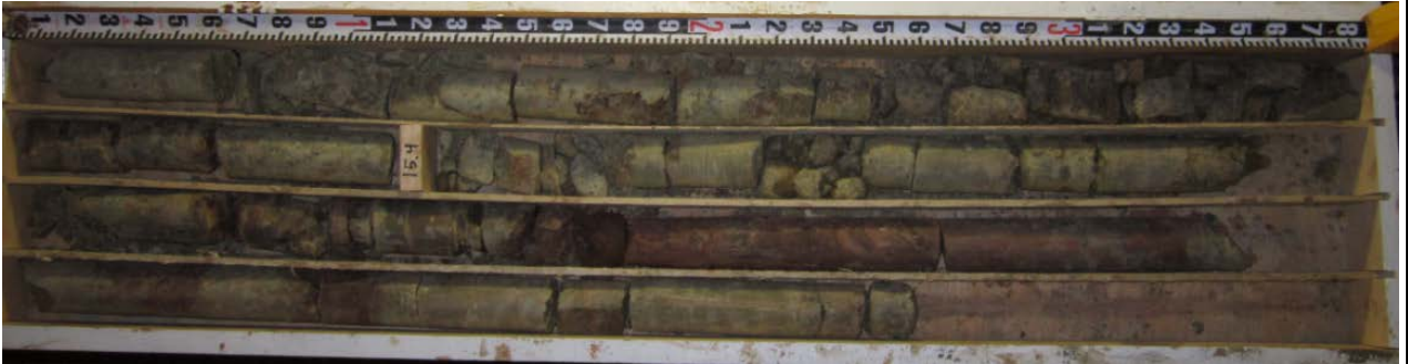
SHP MP 9.3 Boring B-1: Box 1 of 3 (10.4 to 25.4 ft bgs)
