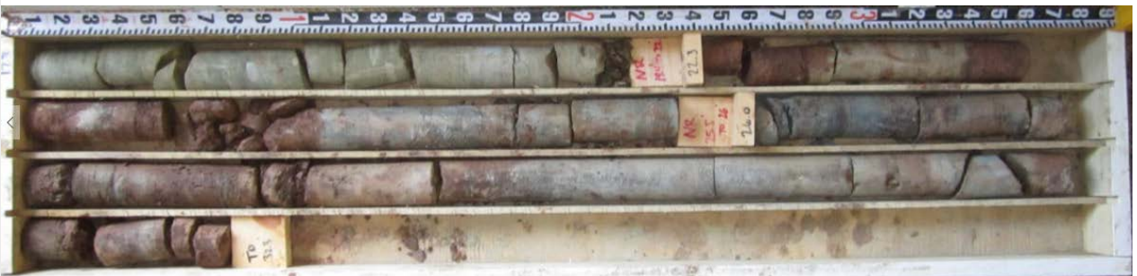
SHP MP 2.8 Boring B-2: Box 1 of 1 (17 to 32 ft bgs)
