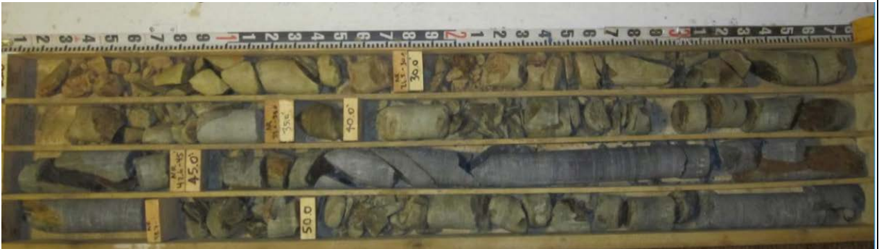
GWNF MP 120.3 Boring B-1: Box 1 of 2 (25.0 to 55.0 ft bgs)
