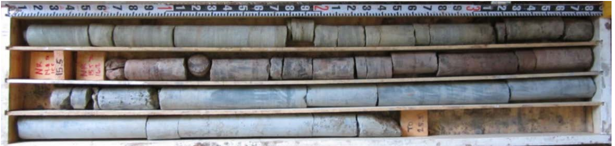
SHP MP 2.8 Boring B-1: Box 1 of 1 (11.0 to 25.5 ft bgs)
