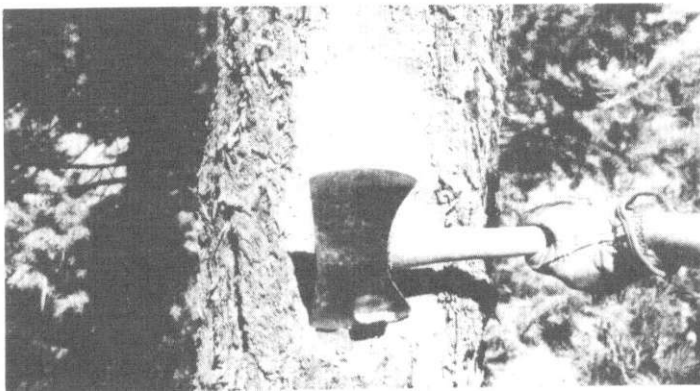
Figure 4-8.--Proper method for blazing a bearing tree. This step is usually left to an authorized land surveyor or crew. A bark knife used in conjunction with a hatchet is also useful and efficient. A clean, concise cut can be obtained by striking the knife. Hearing and eye protection is advisable.
